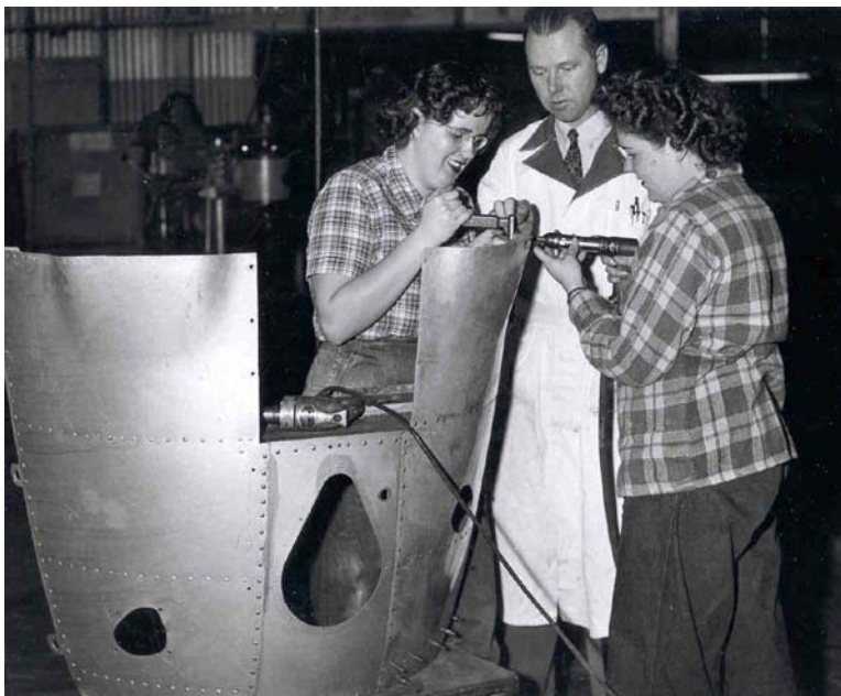
Figure 2-1: “Rosie the Riveters” — women in the Aviation Mechanics Shop, Mel Gaskill, instructor, Eugene Vocational School, c. 1941-1945. The women worked in pairs — the riveter used a gun to shoot rivets through the metal and fasten it together, and the buckler used a bucking bar on the other side of the metal to smooth out the rivets (Source: Lane Archives).
