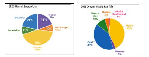
The most current figures at the time of publishing this document indicate that renewable resources account for 11% of Oregon's total energy usage. While we possess robust hydro-electric resources that provide 42% of our electricity load, in and out of state coal-fired power plants still account for a majority of our electrical usage with wind, geothermal and biomass renewables comprising the smallest slivers of Oregon's electricity pie. However, as the remainder of this report will show, the
